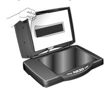
4. Turn the scanner over and slide the lock tab to the unlocked position. The scanner must be unlocked for you to continue with the installation. It must also be unlocked to scan.
